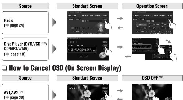
\*1 To switch Operation Screen ON, touch the center of touch panel or press [ENTER] on the remote control.
